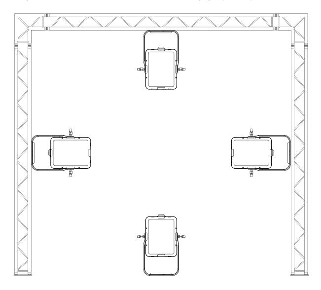
The eLumen8 CYC100 RGBW 100W COB Cyclorama Wash MKII can be operated in a number of mounting positions as shown in the diagram above, hanging upside-down from the ceiling or truss, mounting sideways on truss or stood upright on a flat level surface. Always use a safety wire as an extra safety precaution to prevent damage/injury in the event a clamp fails (see the next page for clamp installation). Never use the carry handles for secondary attachments.
