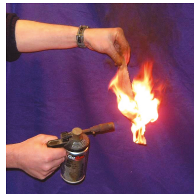
Uncoated fabric under fire conditions
