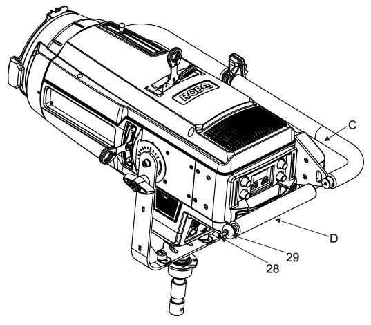
10. Screw the part with weight (E) on the rear side of the T11 fixture by means of two screws with plastic heads (33). Screw the cap (29) back to the rear handle (D) by means of the screw (28).
